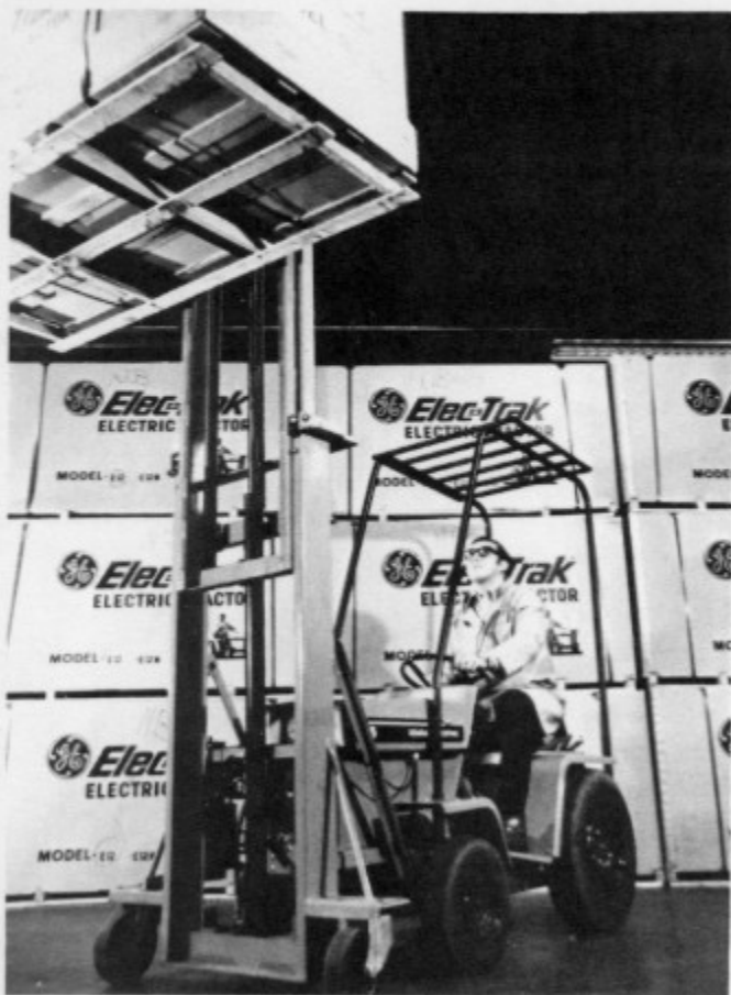
'MIGHTY-MITE' TRACTOR (left) can use telescopic mast to lift 750 lb up to 92-in. high on 36-in. forks. NUMEROUS ATTACHMENTS (upper right) can be applied for a variety of indoor or outdoor jobs—even as front-end loader! TRACTOR PROVIDES POWER (lower right) for vacuum unit, used as a trailer or as a manually-pushed device, on hardened surfaces.
