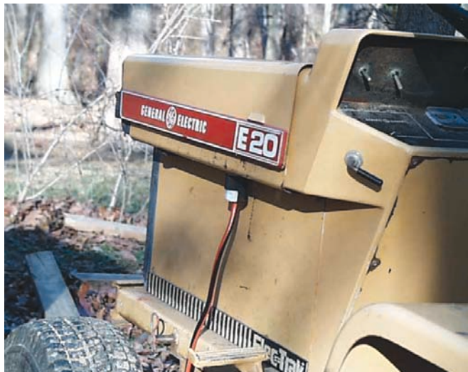
The solar-electric charging system hooks up to the Elec-Trak's 36 volt accessory port.
