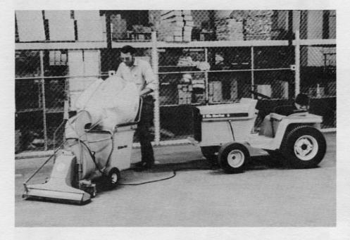
For those hard to reach areas, the compact vacuum system has a hand-operated extension hose which enables your maintenance crew to vacuum areas above floor level and in hard-to-reach corners. All vacuum systems for the Elec-Trak tractor have their own motors, are quickly attached and removed, are operated from the tractor's power and are easily adapted to your particular requirements.
