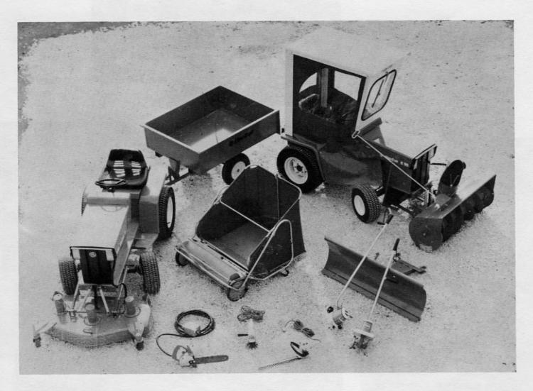
A POWER CENTER ON WHEELS, the versatile Elec-Trak tractor is the heart of a complete groundskeeping system. It will quietly mow around buildings and businesses, finish off up to six one-half acre lawns . . . and take care
