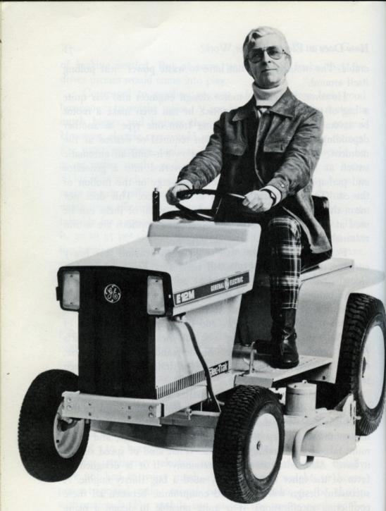
Electric propulsion is also helping to take the noise and fumes out of weekends in suburbia. The E12M Elec-Trak, one of a line of electric tractors, is manufactured by General Electric. This lawn tractor is equipped with a 42-inch mower. It has three forward speeds and two reverse in three gear ranges for a total of nine forward speeds. (General Electric Company)
