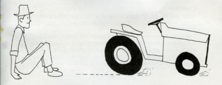
The mower blades stop in less than 3 seconds. When you get back on the seat, the tractor will not restart until the speed control is returned to the neutral position and mower will not start until the P.T.O. is turned "OFF" and back to "ON". Also when the brake pedal is fully depressed, it shuts off the tractor drive motor.
