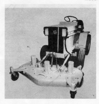
The basic 42" Rear Discharge Rotary Mower is also available with a side discharge option, depending on the Discharge Kit purchased.
