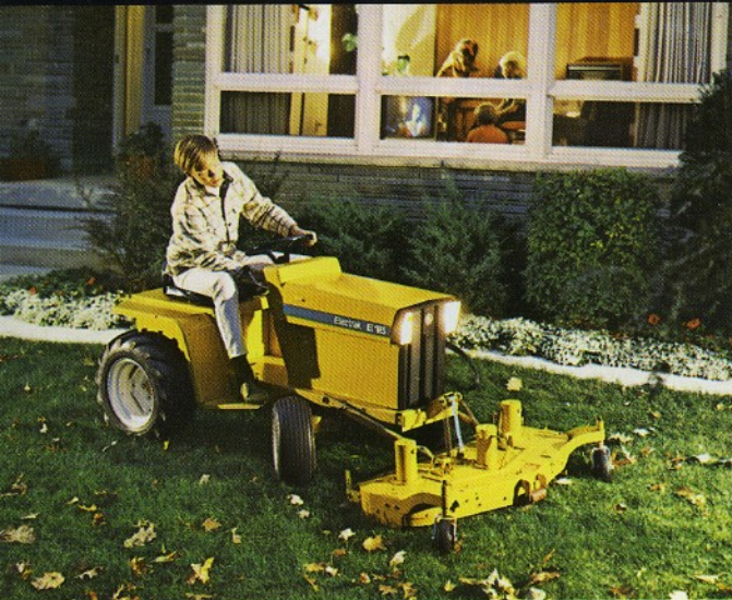
The safer, rear discharge mower allows sweep-up of leaves and grass clippings while mowing . . . and the front mounting lets you trim close.
