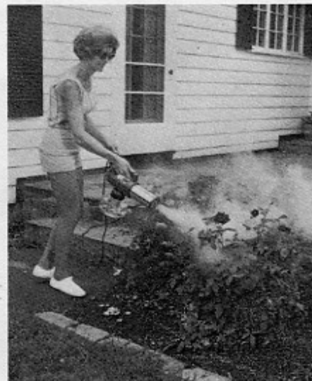
Garden fogger runs off the tractor's 36-volt powerpack, too. The low-voltage power system is well below the shock-hazard level.
