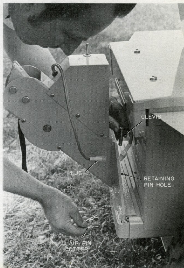
Figure 1. Rear Electric Lift Installation
