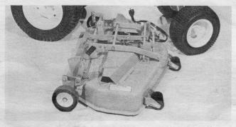
Fig. 2. Position Mower to Right of Tractor
