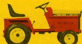
EGT-150 (16-hp Class) Electric Garden Tractor offers either 42" front- or mid-mounted mower, electric accessory lift, "Power Pulse" for extra surge of power.
